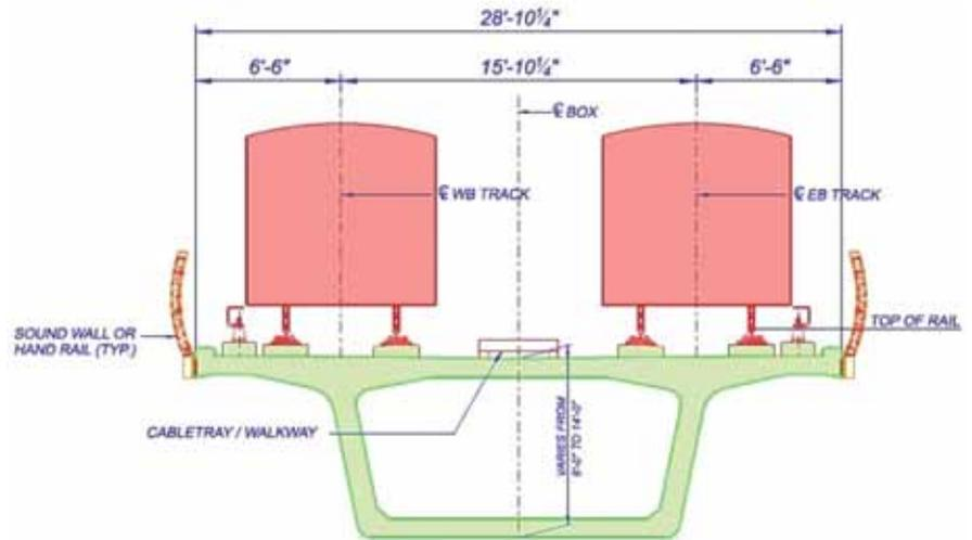
Typical section through the dual-track segmental box girder. Drawing: URS Corporation.
